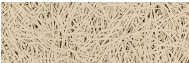
Fibre width 2 mm, characteristic surface
