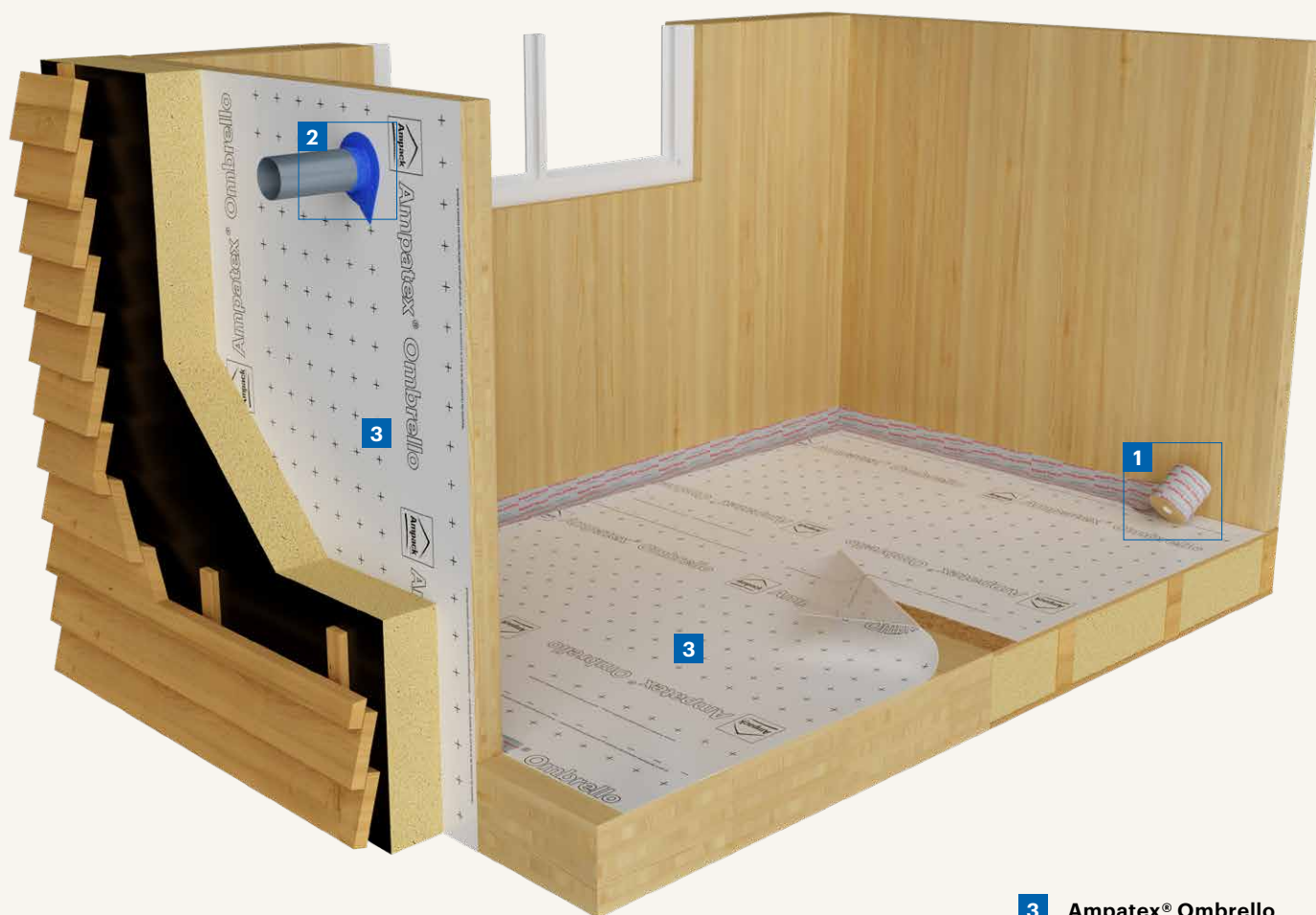
3 Ampatex® Ombrello Weather protection / construction period cover, fully self-adhesive
